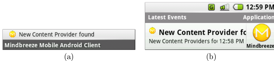
Figure 6.12: Android client status bar notification (a) and pull down menu for navigating to the action intent of the notification (b)
